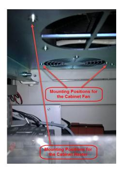
The heater and the fan are held in position by 2 rivet nuts each, as highlighted in the picture.
