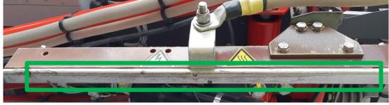
If there are a few arc spots, grind the rails and recommended to swap the rails diagonaly.
